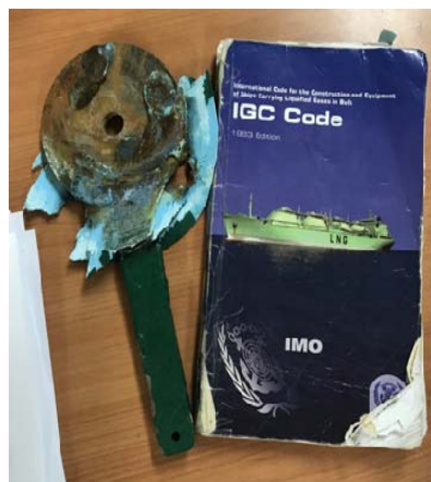
Figure 3 – (left) Orifice plate temporarily removed to clear debris from deck water spray system. Note approx 2 inch internal diameter of pipe reduced to 1/2 inch trapping most debris behind each plate. At least 9 orifice plates were identified on this VLGC. Photo Credit – Mr. Jamie Wilson USCG Sector Houston-Galveston
