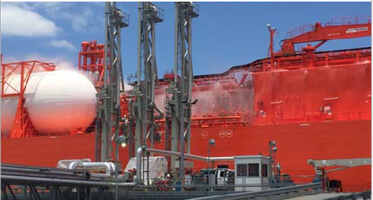
Figure 6 – Testing of deck water spray during an initial COC-Gas Exam conducted in Houston, Texas.
